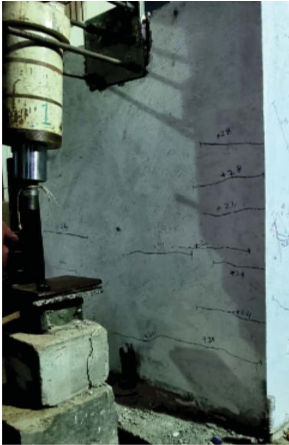
Fig. 19 Failure crack pattern S-02 (left)
