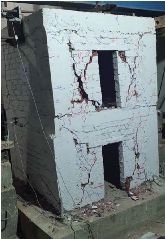
Fig. 11 Crack failure pattern S-01 (back)
